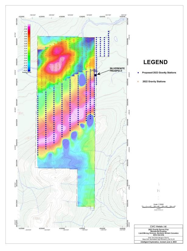
**Figure 1. Location of Gravity Stations for the 2023 Survey – Silverknife Property** (Source: McKeown Exploration Services)
