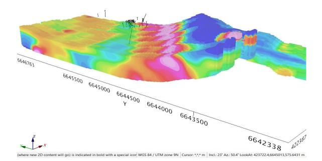
**Figure 4. Conductivity 3D Geonic Model Looking in a Westerly Direction – Silverknife Property** (Source: Intelligent Exploration)
