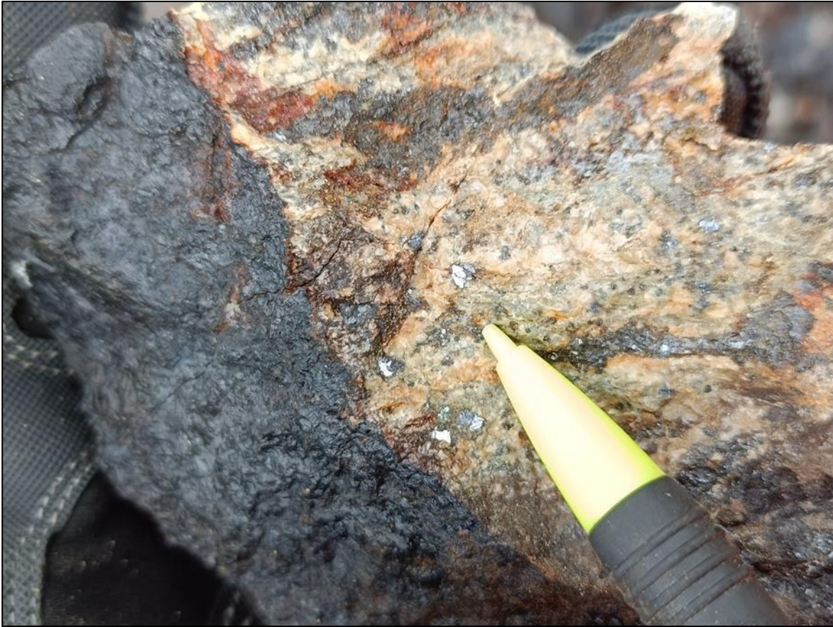
Plate 3: Hand sample collected from the 4450 level dump, massive sulfides in contact with intrusive with disseminated galena
